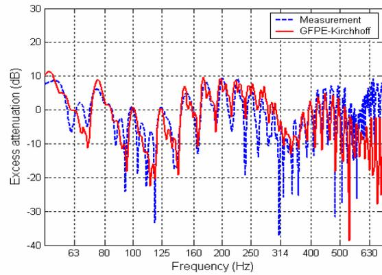
**Figure 3:** Comparison between GFPE and scale model measurements for the configuration detailed in Figure 1,  $c(z) = c_0(1 + 4.9 \times 10^{-3} z)$ ,  $\sigma_{barrier} = 180$  cgs .
