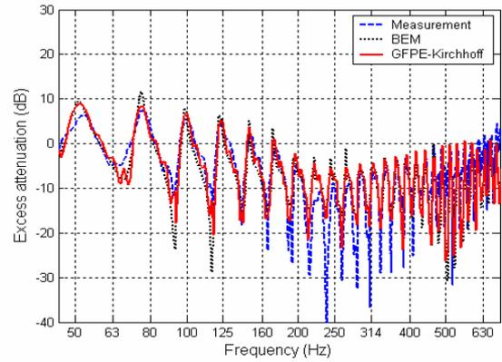
**Figure 2:** Comparison between GFPE, BEM and scale model measurements for the configuration detailed in Figure 1,  $c(z) = c_0$ ,  $\sigma_{barrier} = 180$  cgs
